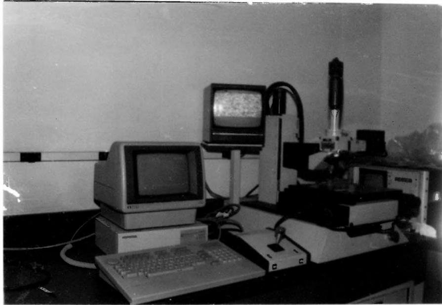
Fig. 5.4 Photo of matrix videometric microscope
