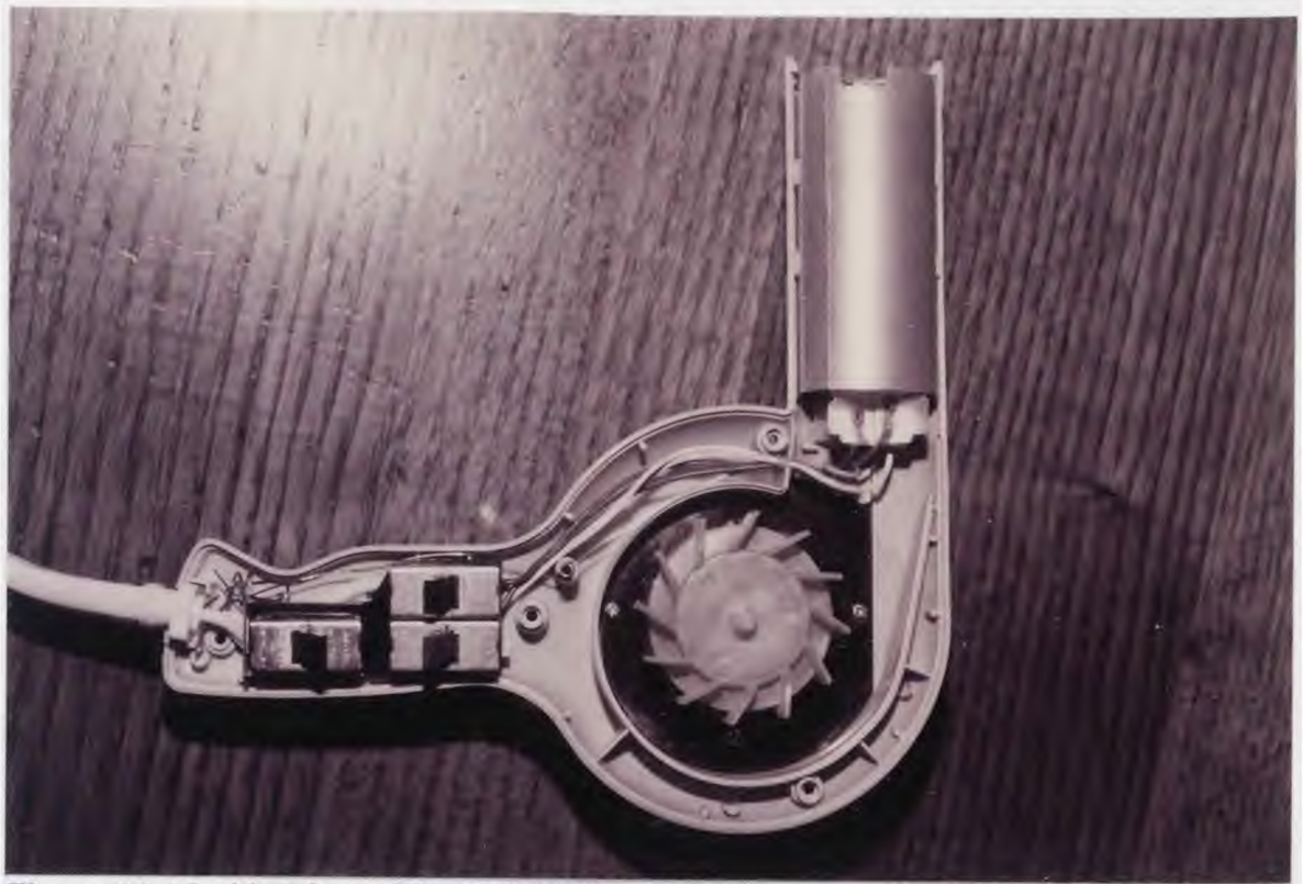
Figure 13.1 Inside View of Hand Held Hair Dryer
