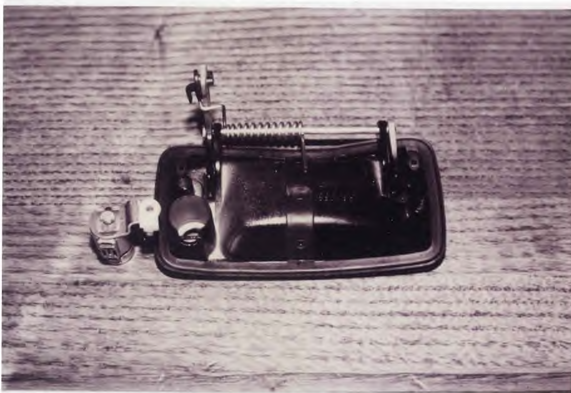
Figure 10 Car Door Handle Assembly With Lock Sub-Assembly
