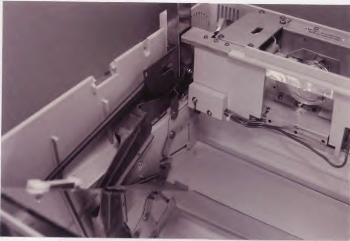
Figure 9.3 Inside View of the Projector Showing Mirror, Linkage, Elevator and Column
