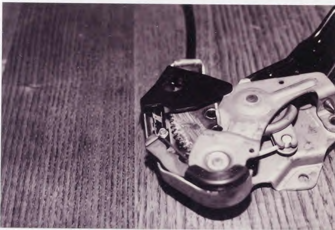
Figure 8.2 View of the Emergency Brake Ratchet Sub-Assembly
