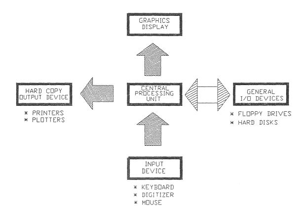
Figure 7. A Typical CAD System
