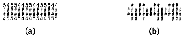
Figure 5.1 A fuzzy image and the corresponding binary image by an \alpha -cut with \alpha = 0.5 .
