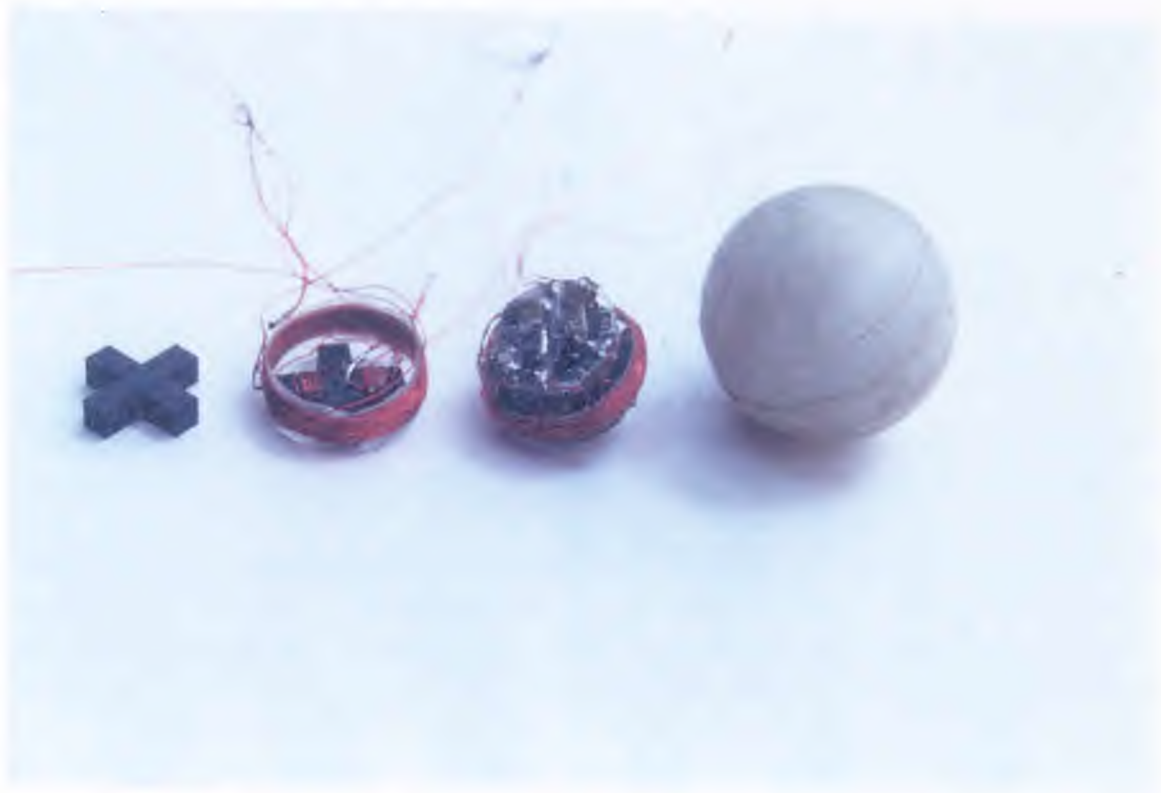
Figure 2.4 Exploded View of 3 Transmitter Assembly
