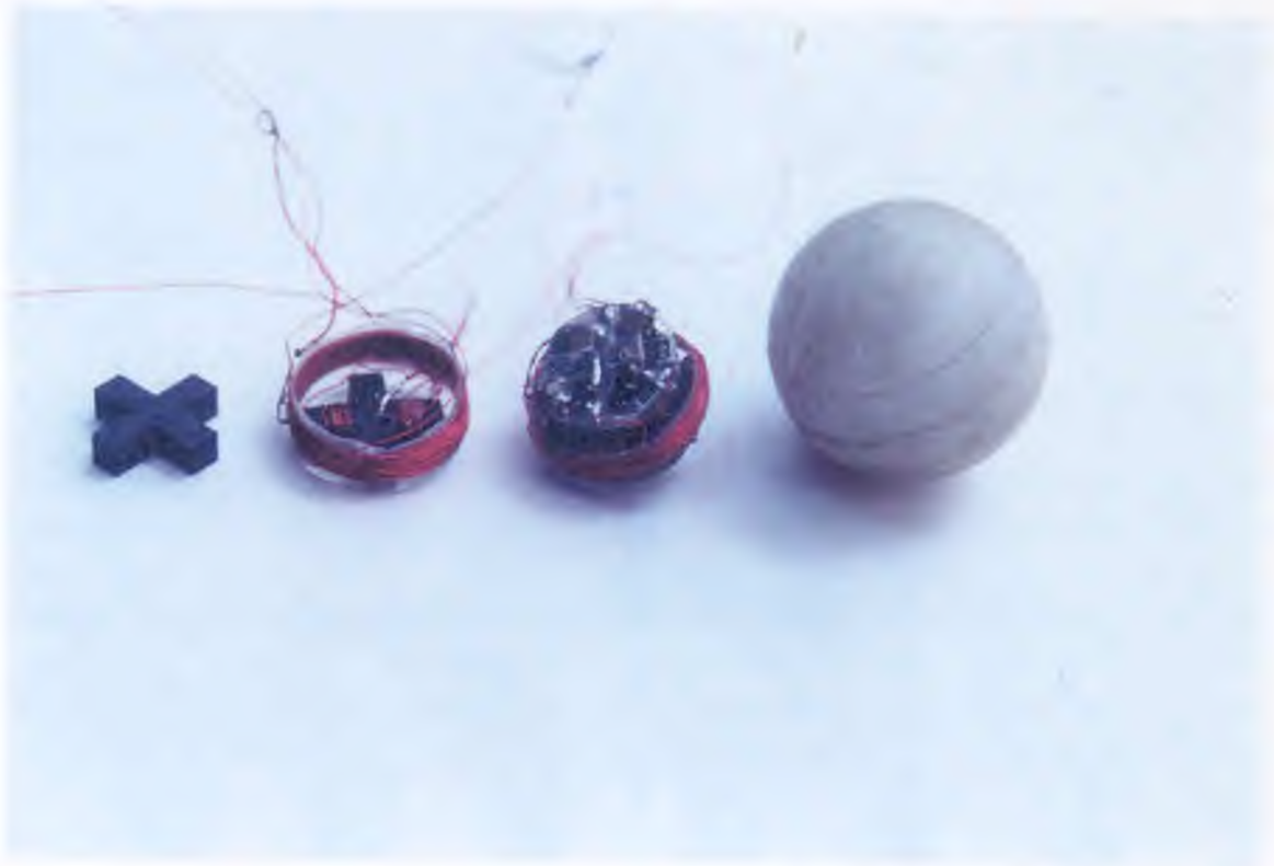
Figure 2.4 Exploded View of 3 Transmitter Assembly
