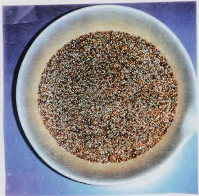
Pellet Injected through Pneumatic Injection System (50 psi)
