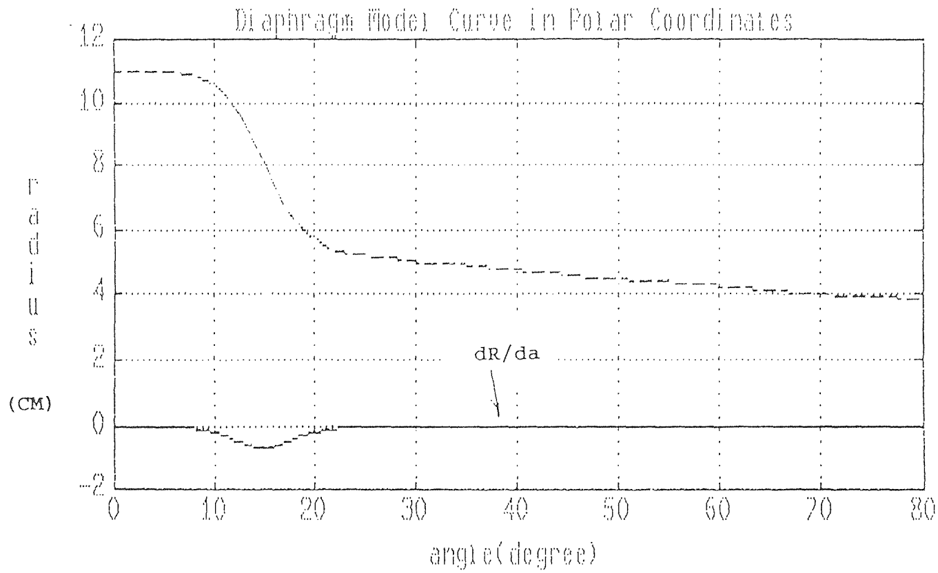
Figure A.3 Diaphragm model curve in polar coordinates while r_0=11\text{cm} , t_e=0.3\text{N/cm} .
