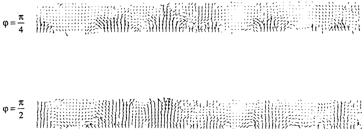
Figure A5.11a Mean velocity fields for phases \pi/4 ( y_b = 0.0359\text{m} , v = 1.58\text{ m/s} ) and \pi/2 ( y_b = 0.05\text{ m} , v = 0 ). (Primary computational cell dimensions \text{length} \times \text{width} = 100d \times 1d )
