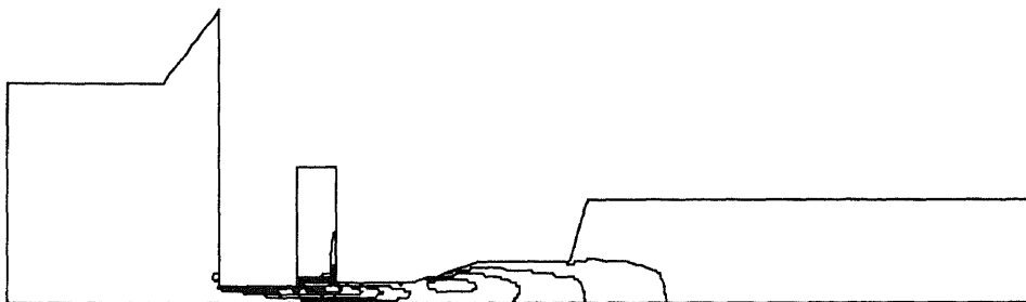
Figure D.2 Turbulent Kinetic Energy Contour for Pulsed Nozzle (Contour Level: k_{\max} = 0.249 \times 10^9 \text{ cm}^2/\text{s}^2 and k_{\min} = 0.160 \times 10^4 \text{ cm}^2/\text{s}^2 ) at t = 0.5 \times 10^{-3} sec After Initiation of the Pulsate Flow; (Test conditions are identical to those in Fig. D.1).
