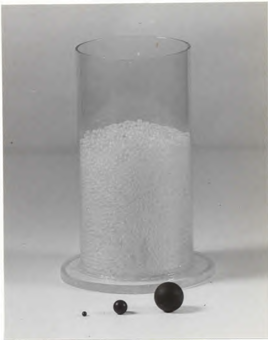
Figure 5 Experimental cell and material used for vibratory experiments.
