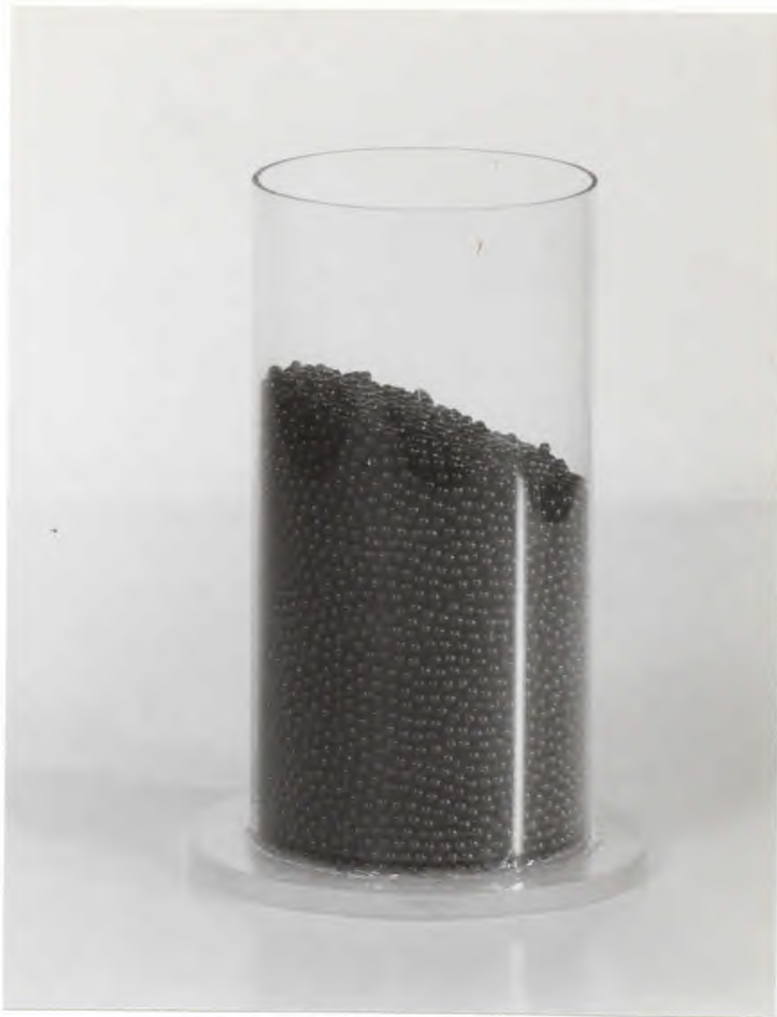
Figure 1 Cylindrical setup for the determination of the angle of repose by pouring .
