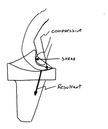
Resultant Force for Tibial Component of the Insall-Burstein
