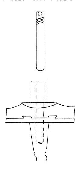
Front Loading Tibial Insert with Dovetail/Pin
