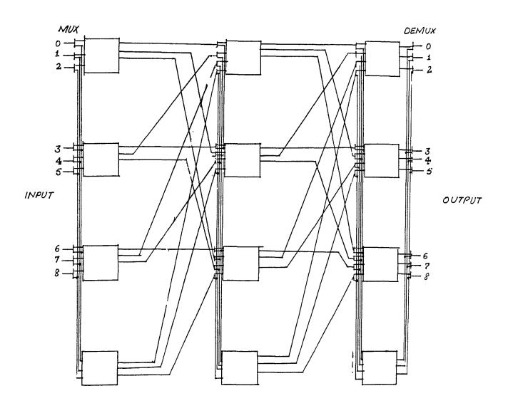
Figure 3.2:  $9 \times 9$  FTC network with one extra switch per stage.
