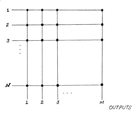
Figure 1.3:  $N \times M$  Crossbar switch
