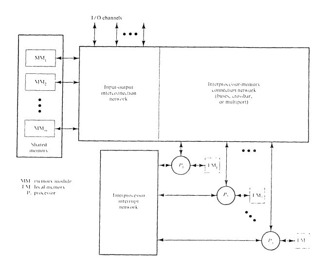
Figure 1.1: Functional Design of a Multiprocessor System
