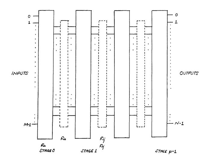
Figure 2.2: A generalized multistage interconnection network
