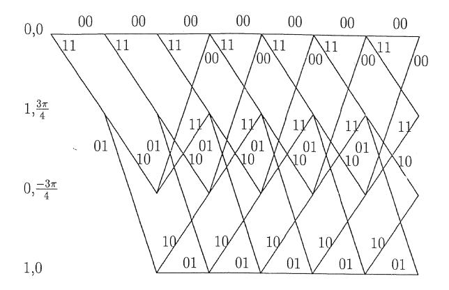
Fig. 7. Trellis of combined coding and TFM modulation for the encoder [1 + D, 1] with R = 1/2, v = 1.
