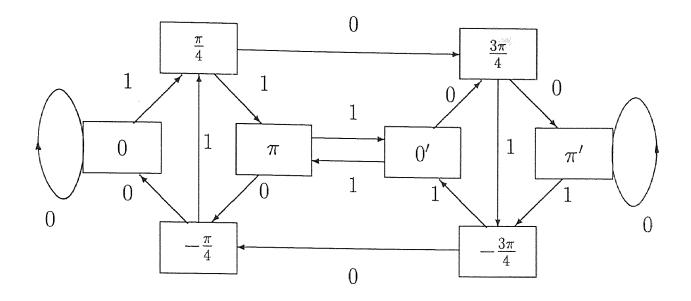
Fig. 3. The finite state machine of TFM modulation. The branches are labeled by the input bits to the TFM modulator.
