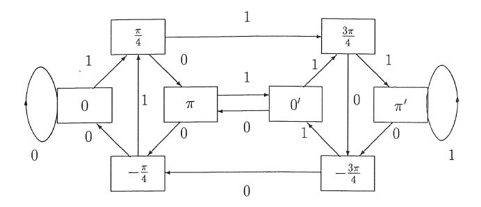
Fig. 5. The finite state machine of precoded TFM modulation. The branches are labeled by the input bits to the precoded TFM modulator.
