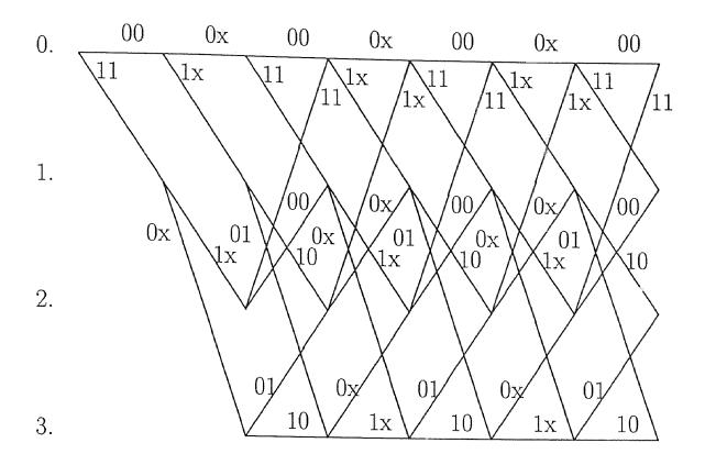
Fig. 9. Trellis diagram of R = 2/3, v = 2 code produced by periodically deleting bits from R = 1/2, v = 2 code of Fig.8. x is a deleted bit.
