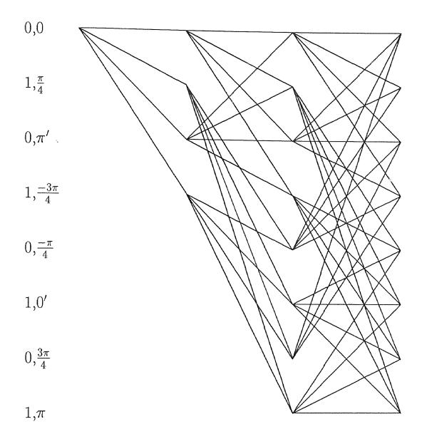
Fig. 12. Trellis diagram (original) of combined coding and modulation of encoder [1 + D, 1, 1 + D] with R = 2/3, v = 1.
