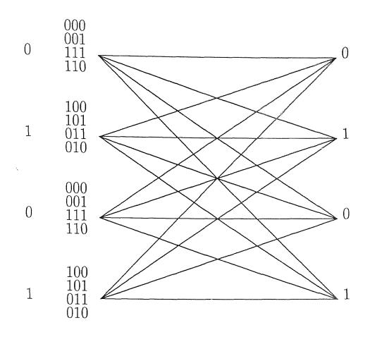
Fig. 10. Trellis diagram of the punctured trellis encoder [1 + D, 1, 1 + D] with R = 2/3, v = 1.
