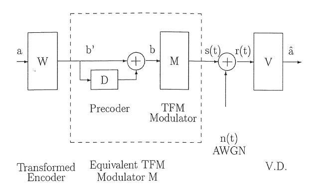
Fig. 4. Combined coding and precoded TFM modulation communication system model.
