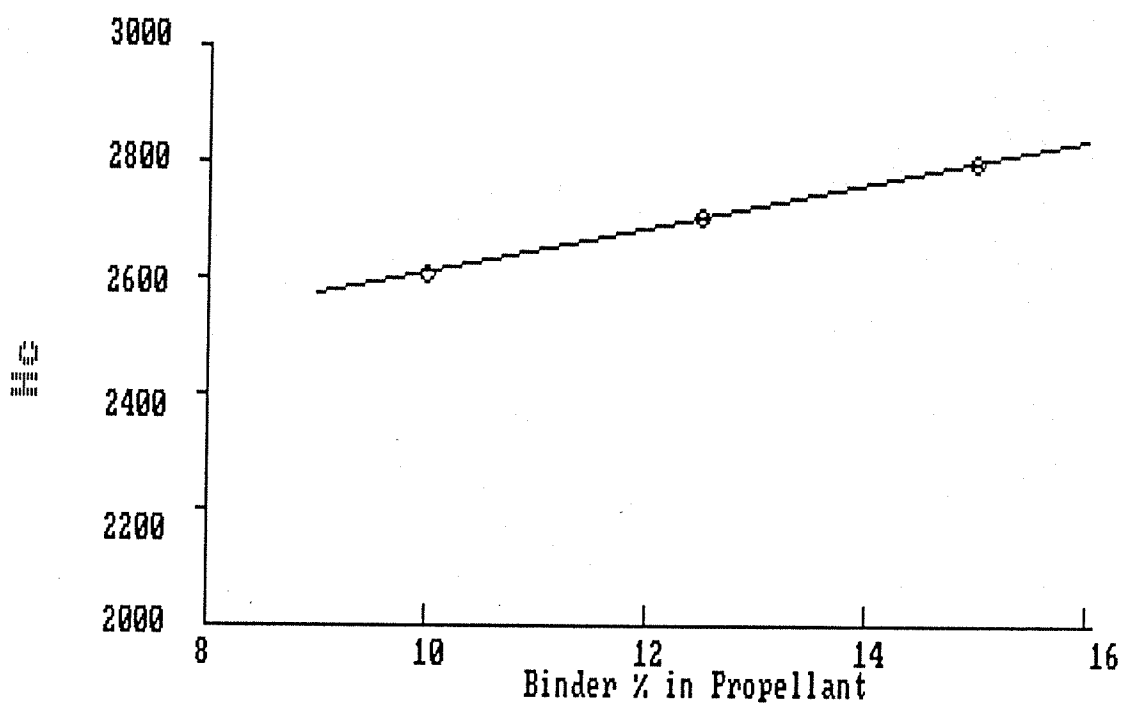
Fig 28. Effect of binder % in propellant on \Delta H_C
