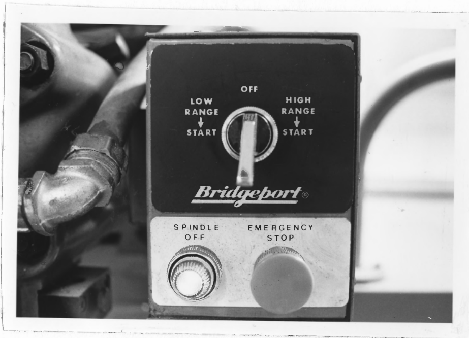
Figure 5-2 Spindle Control Panel
