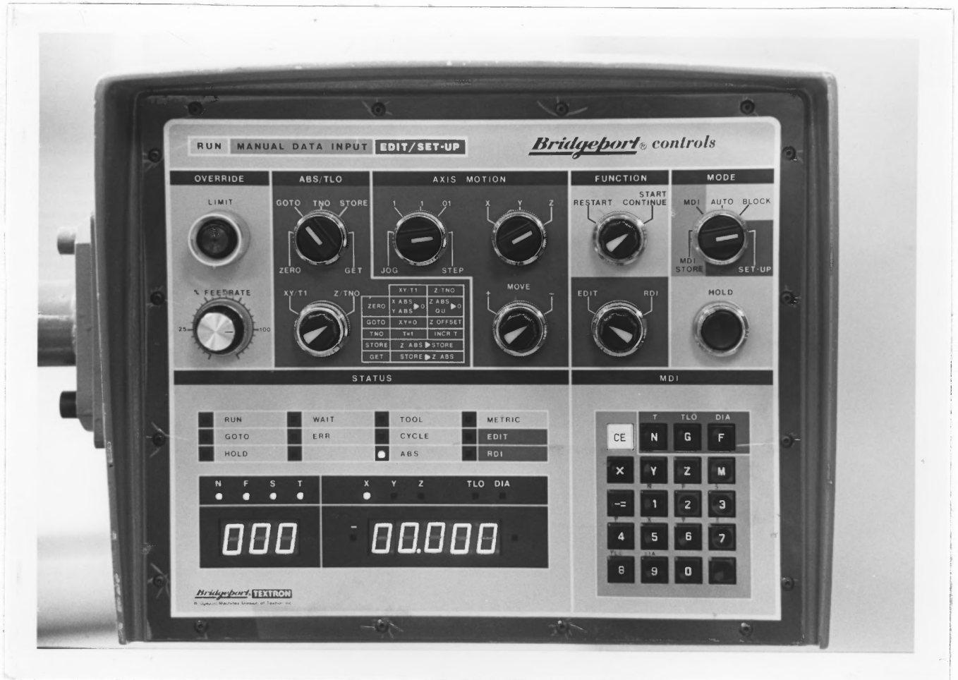
Figure 5-1 Operator's Main Control Panel
