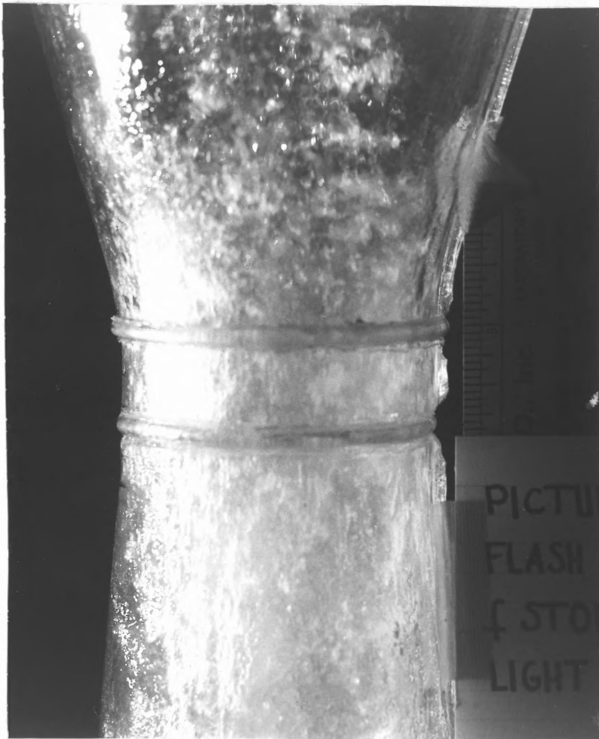
Figure 7.6 Photograph taken with Minolta SRT-201 camera and Vivitar 285 flash at yellow mode on Kodak Plus-X film (side lighted, flash at 1 ft, f/11)
