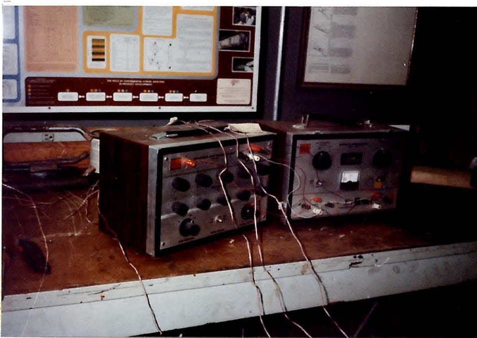
FIGURE 2.6.b STRAIN GAUGE INDICATOR
