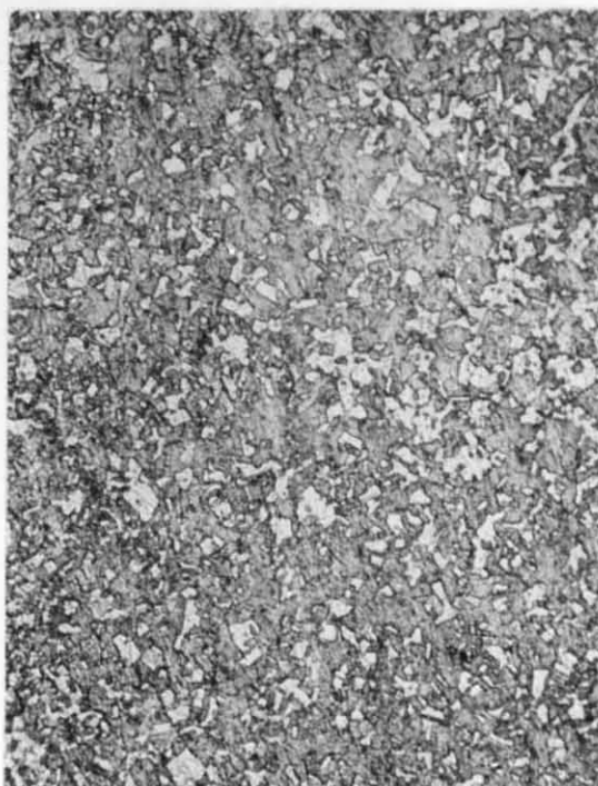
(b) Stressed to 33ksi at 250 deg F for 9.2 hours. Approximately 3 in. from fractured surface.
