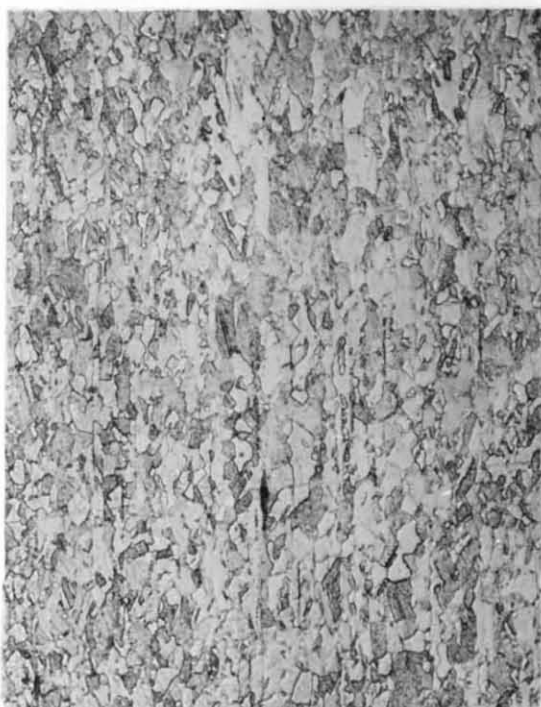
(b) Stressed to 33ksi at 250 deg F for 9.2 hours. Approximately 3 in. from fractured surface.
