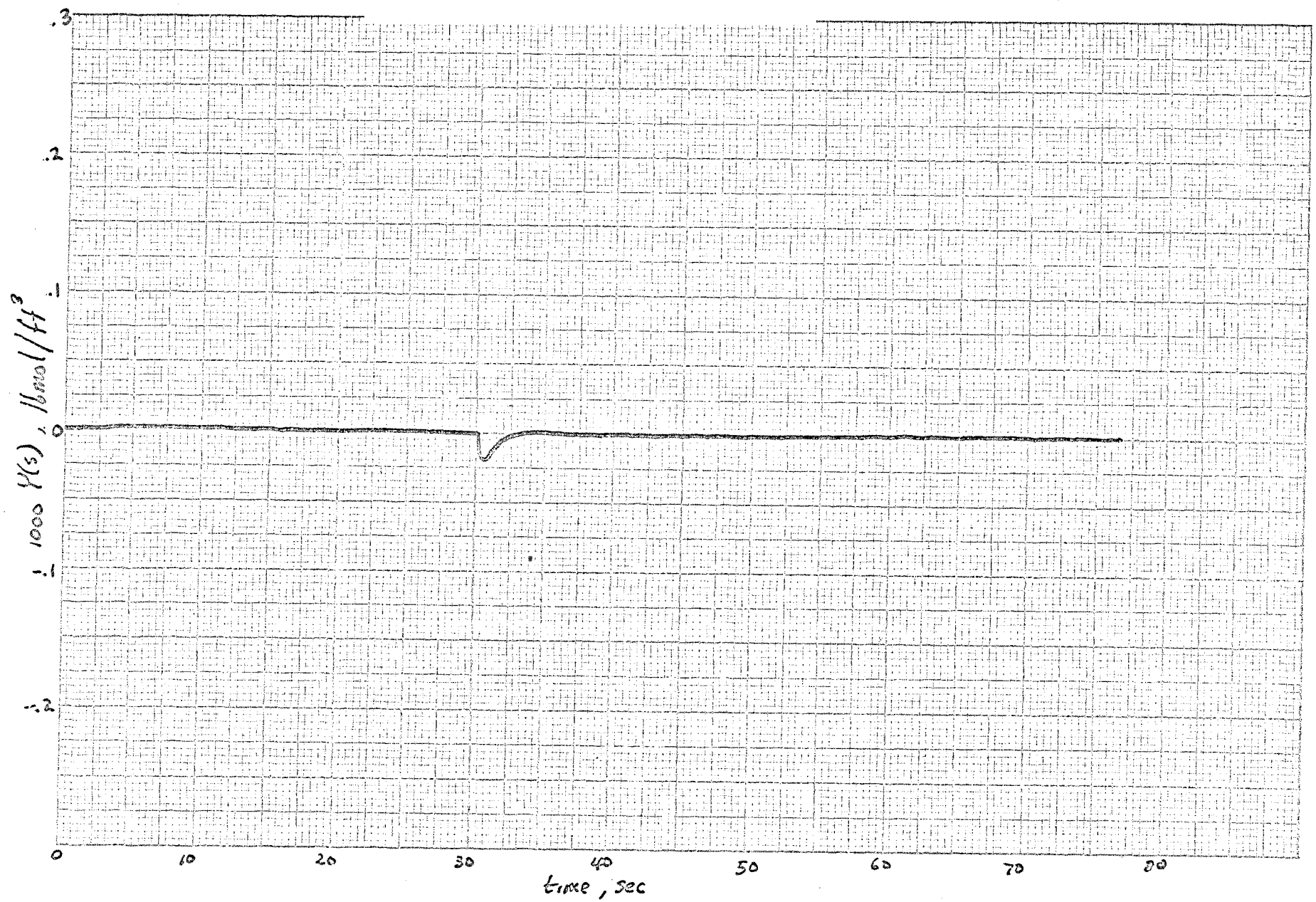
Figure 27 TRANSIENT Response for Feedforward-feedback Control, PID: K_c=4, \tau_I=.1, \tau_D=10 Change in load.
