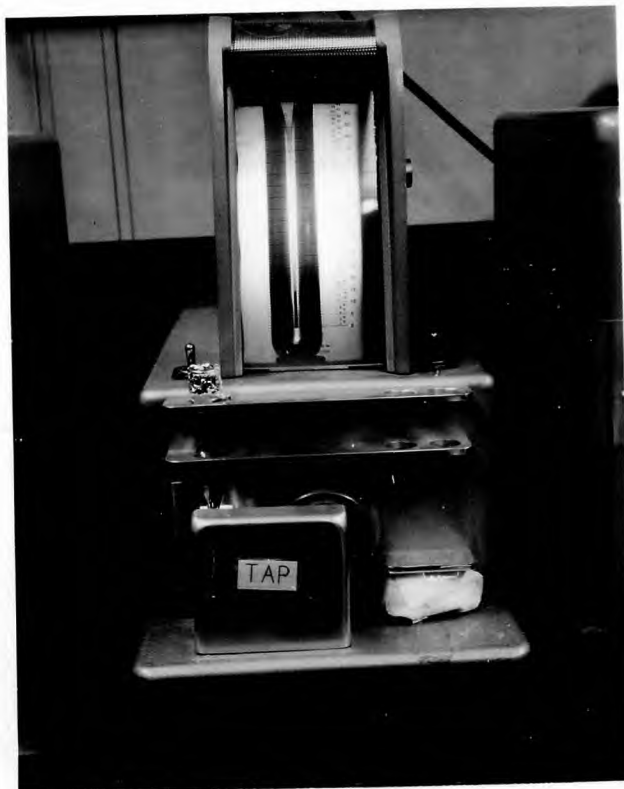
FIGURE 6. CENTRIFUGE TUBE IN PROJECTOR FOR READING OF SEDIMENT HEIGHT
