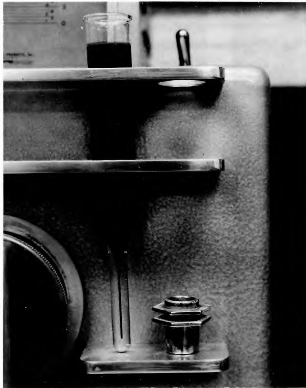
FIGURE 4. FEEDING CHAMBER AND CENTRIFUGE TUBE Tube has been filled with ink to show inside contour. Note the line at top of the ink level, to which sedimentation liquid has been filled.
