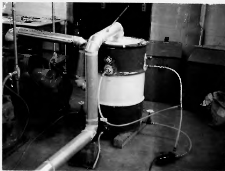
Rear view showing mixing barrel, turbo-blower and cooling water pump.
