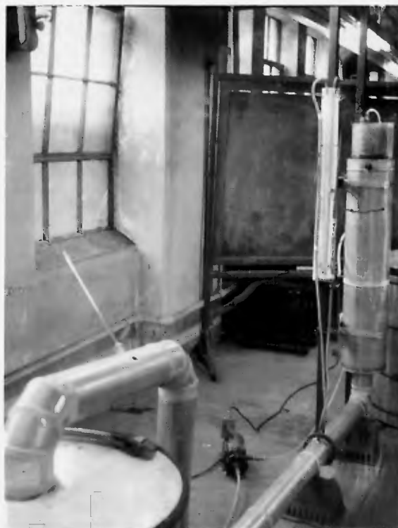
Side view showing test column, orifice plate, manometer, and nozzle water pump.
