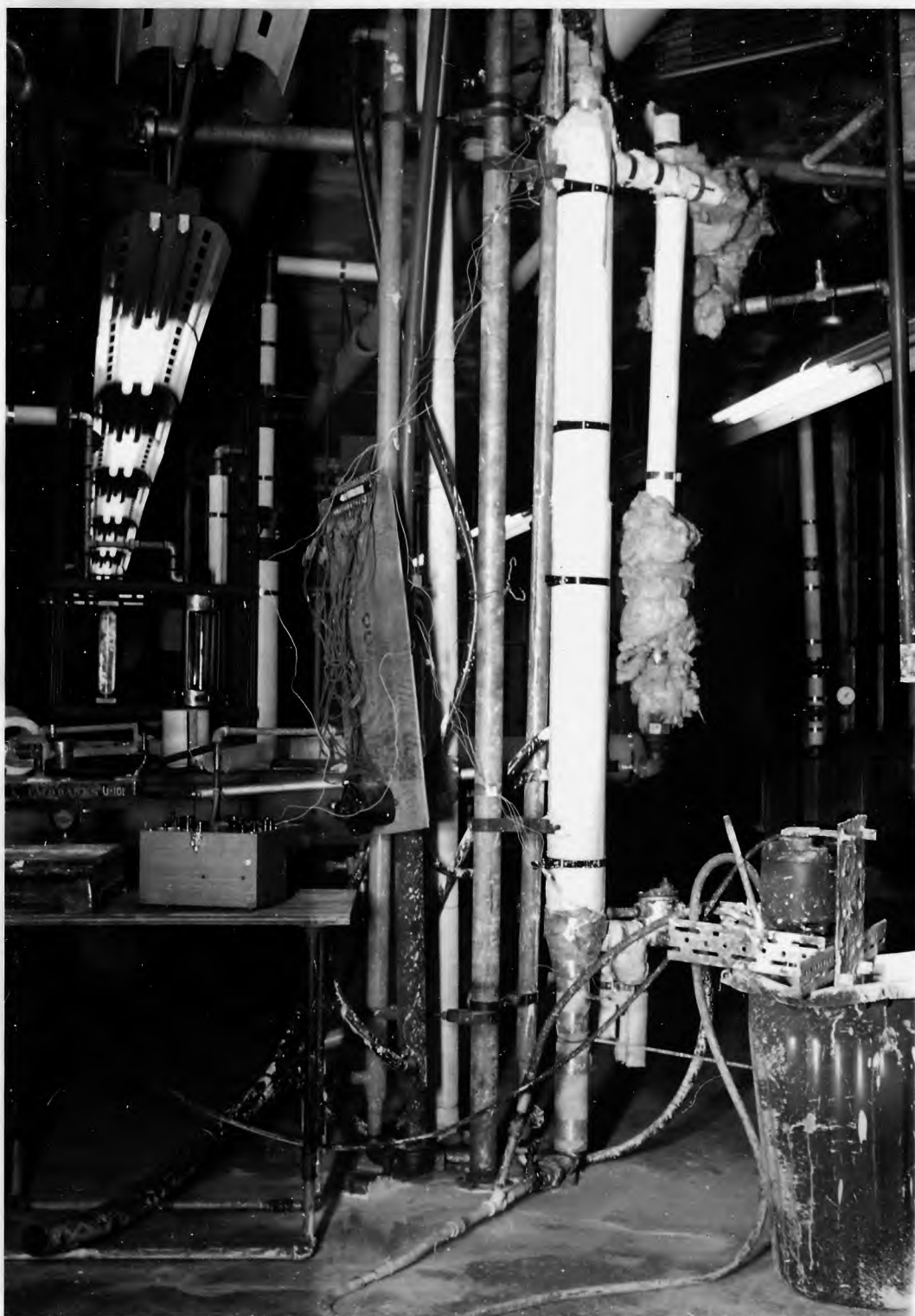
Figure 2a View of apparatus showing heat exchanger, coolers, potentiometer, multipoint thermocouple switch, and slurry storage tank with submerged circulating pump.
