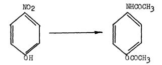
The reaction mixture was prepared as before, and 0.1 mole of para-nitrophenol was added. The mixture was heated at reflux until a clear solution was obtained (about 10 minutes). Approximately one-half the volume of liquid had been distilled when crystallization began to take place. The distillation was stopped and the flask placed in the refrigerator over night. The next day there was a mass of crystals which were filtered without vacuum. The crystals were transferred to a beaker and 50 ml. of
