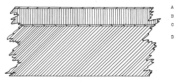
A - Redeposited copper on surface of disk.
