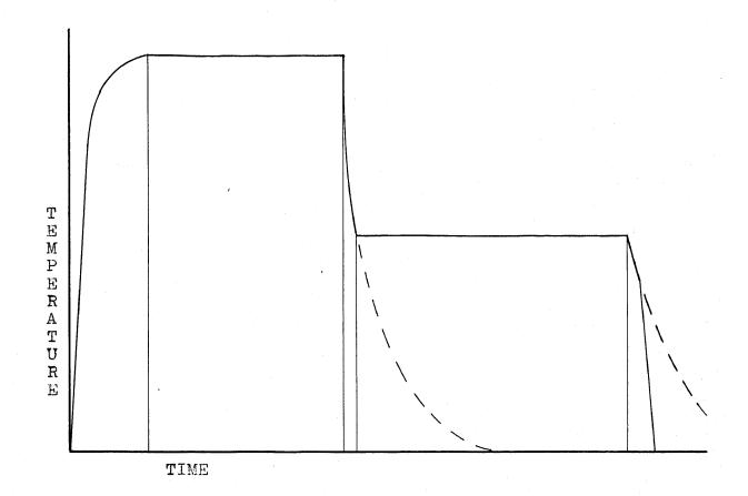
A Temperature-Time cycle for producing disks.
